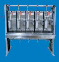
3 Line Wall Mount Rack with cation conductivity columns and cells mounted side by side (analyzers mounted in sample room).
